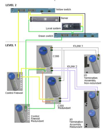
Figure 5: Series C I/O and C300 topology
