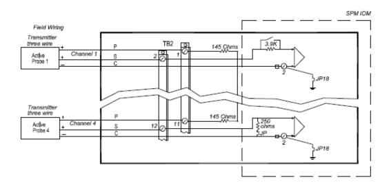
Figure 65: Series C SPM - Active Probe Field Wiring
