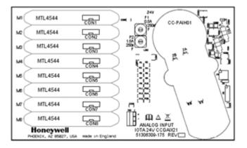
Figure 245: CC-GAIX21 Analog Input IOTA
