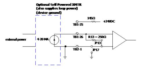
Self-powered 3-wire transmitter (system ground)
