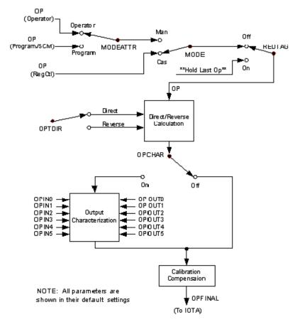
Figure 191: Analog Output conversion
