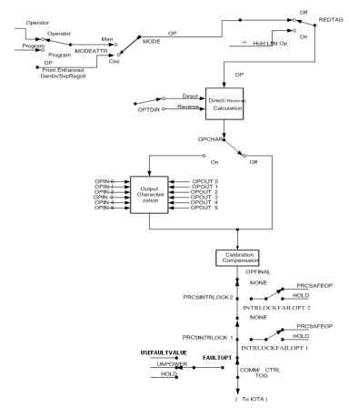
Figure 209: SVP - AO block execution diagram when OPACTION is 'FullValue'
