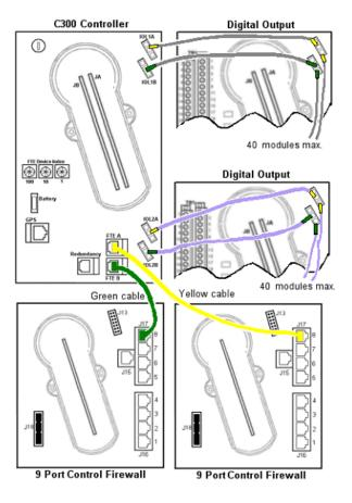
Figure 9: Series C board connections
