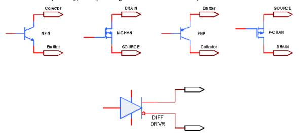
Figure 100: Field device output stage types
