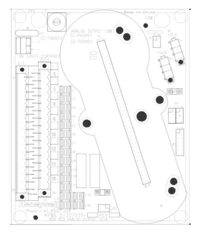
Figure 31: Series C Analog Output 6 inch, non-redundant IOTA
