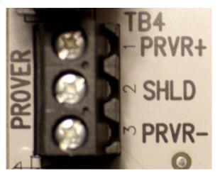
Figure 113: Prover Bus connector - TB4
