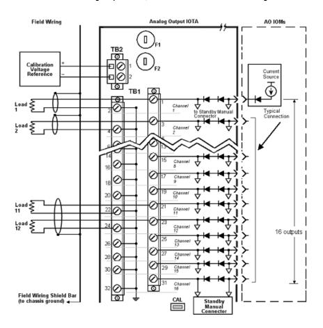
Series C Analog Output 12 inch, redundant IOTA is displayed:
