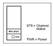
Figure 266: Digital Output - MTL4521 isolator LED indicators
