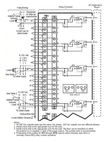
Figure 60: Series C Digital Output Relay Extender board and field wiring connections
