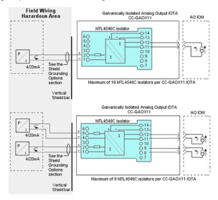
Figure 251: CC-GAOX11 Analog Output IOTA connection diagram
