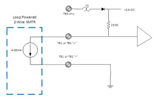
Figure 76: Standard 2-wire transmitter with UIO
