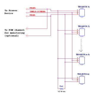
Figure 111: Multiple IOTAs connected in parallel on the Prover Bus
