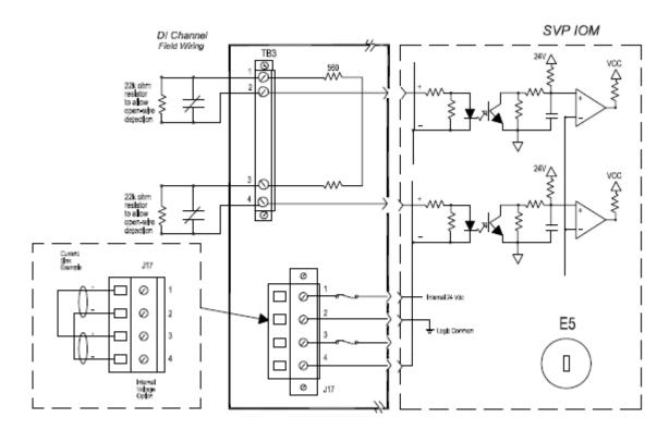
Figure 72: Series C SVP - DI channel Field Wiring
