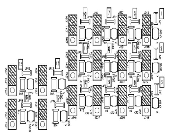
Figure 26: Series C differential non-redundant Analog Input 9 inch, jumper configuration
