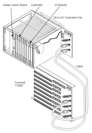
Figure 1: View of existing Basic Controller and Extended Controller
