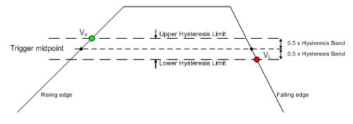
Figure 122: Illustration of upper and lower trip points and hysteresis band
