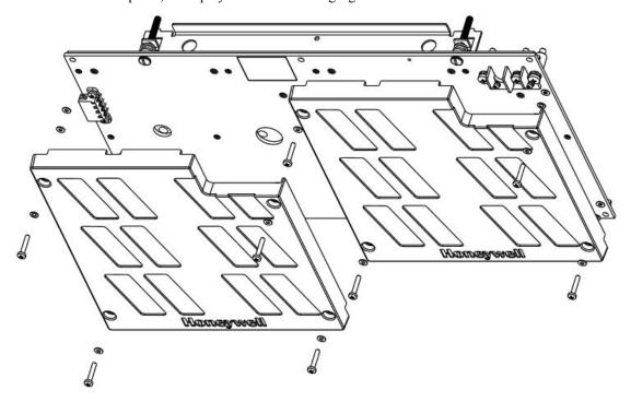
Figure 136: Half panel cover installed on the Backplane
