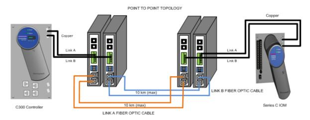
Figure 233: Single mode fiber optic topology
