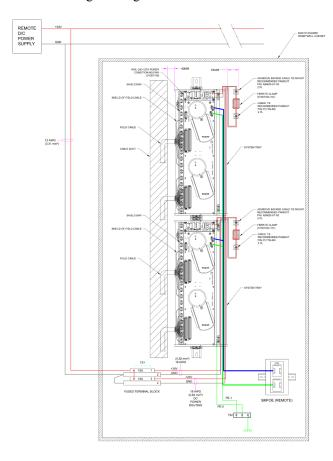
Figure 165: DC power line wiring through system tray
