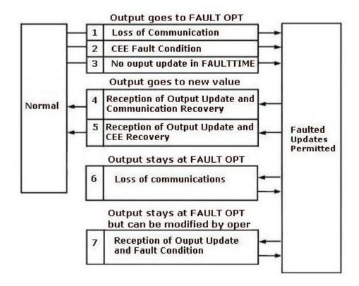
Figure 188: AO and DO fault state (FAULTST) transitions
