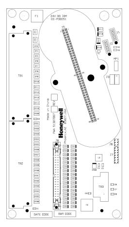
Figure 54: Series C 24V Digital Output 9 inch, non-redundant IOTA
