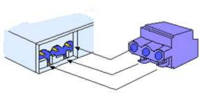
Figure 242: Inserting the terminal plug into the isolator
