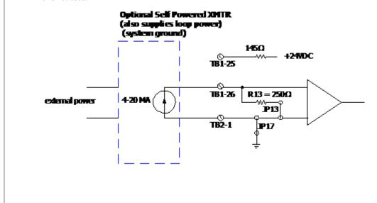
Self-powered transmitter with device grounded
