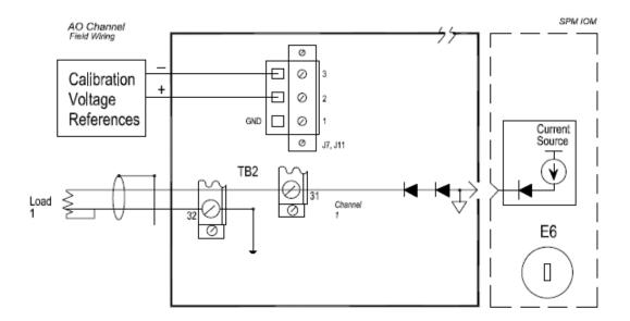
Figure 67: Series C SPM - AO Channel Field Wiring
