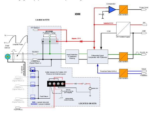
Figure 99: PIM connectivity block diagram
