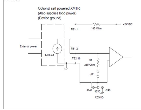
Self-powered 3-wire transmitter (system ground)
