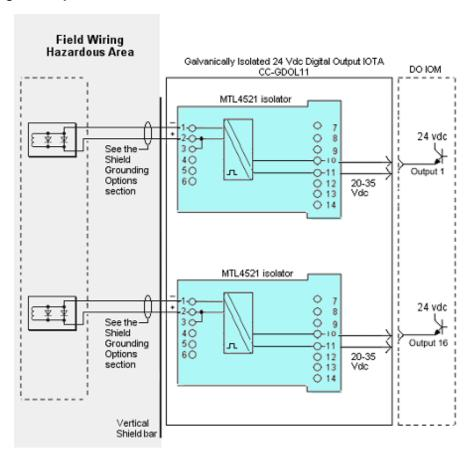
Figure 263: CC-GDOL11 Digital Output IOTA assembly layout
