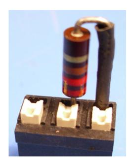
Figure 102: Recommended way of insulating resistor leads and bending them
