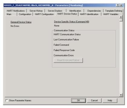
Figure 180: HART Device Status tab
