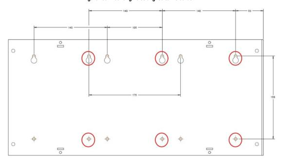
Figure 154: Mounting holes aligned to 10-slot rack
