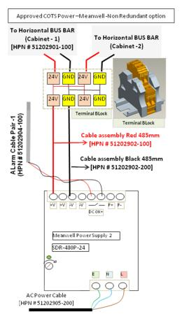
The following diagram displays the connection diagram for COTS Power Meanwell non-redundant system.
