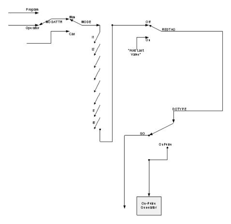
Figure 201: Speed Digital Output conversion
