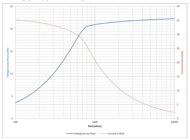
Figure 112: Graph of Prover Pulse voltage and current verses Rext
