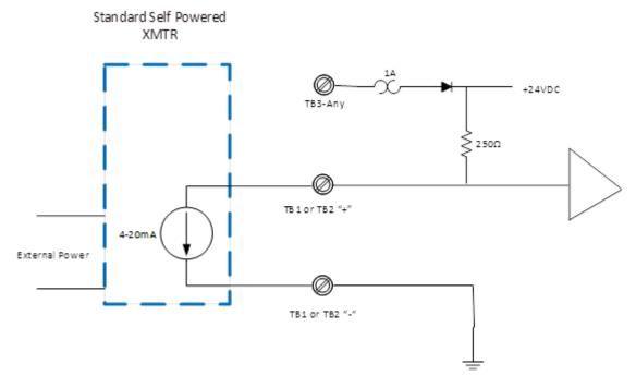
Figure 78: Self-powered 4-wire transmitter with UIO
