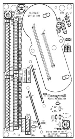
Figure 42: Series C 24V Digital Input 9 inch, non-redundant IOTA
