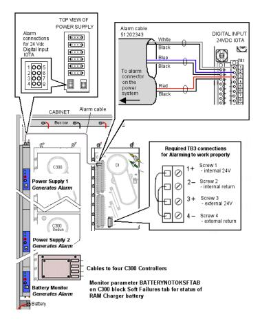
Figure 50: Alarm cable connection to the power supply and 24V DI IOTA for RAM Charger Assembly 51199932-200
