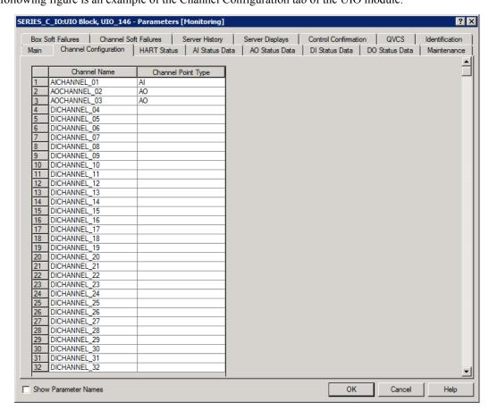
Figure 176: Channel Configuration tab
