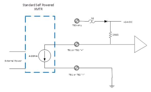
Figure 90: Self-powered 4-wire Transmitter with UIO-2
