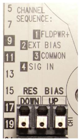
Figure 101: RES BIAS Terminal Block (channel 1 shown)
