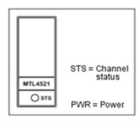
Figure 264: Digital Output - MTL4521 isolator LED indicators
