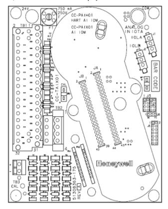
Figure 12: Series C Analog Input 6 inch, non-redundant IOTA
