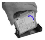
Figure 268: Removing a module from an IOTA
