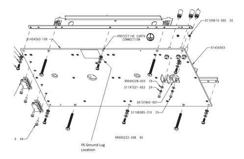
Figure 157: UHIO backplane showing Protective Earth connection
