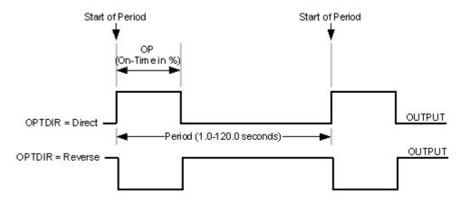
Figure 195: Pulse Width Modulated Output
