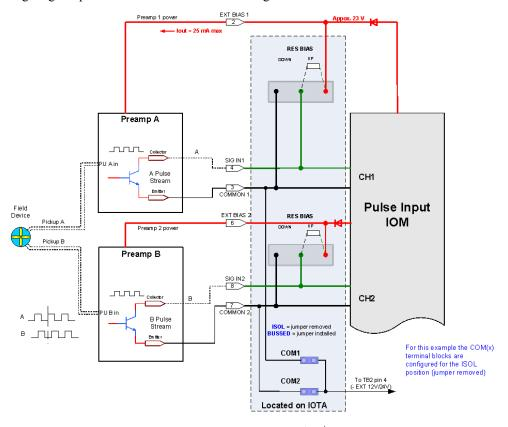
Figure 119: Connecting PIM with dual stream devices
