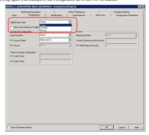
Figure 177: Configuration tab - UIO-DI channel
