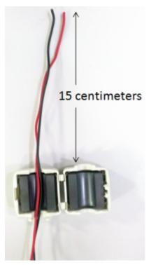
**b** Place the power cables on the ferrite clamp as shown in the following figure.
