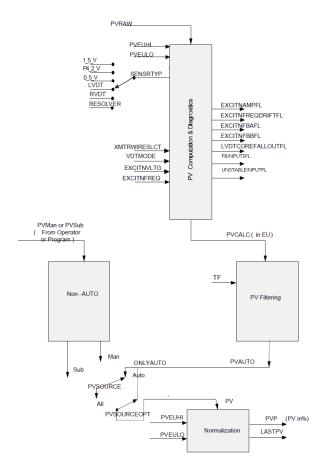
Figure 205: SVP -AI PV processing when it is configured for LVDT or RVDT or Resolver
