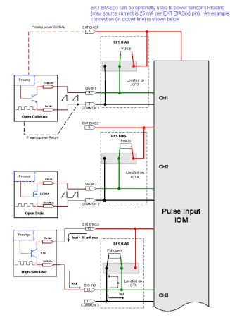
Figure 120: Connecting PIM with other sensor types
