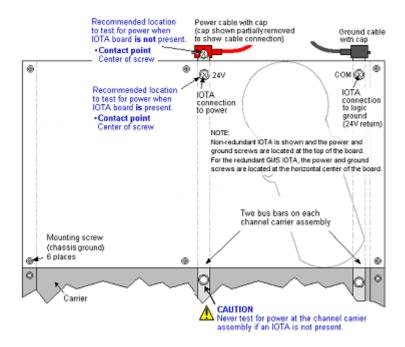
Figure 238: GI/IS Grounding and power connections
