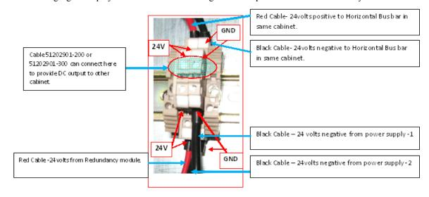
The following figure displays the terminal block wiring for COTS power Phoenix non-redundant system.
