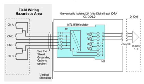
Figure 261: CC-GDIL21 Digital Input IOTA connection diagram
