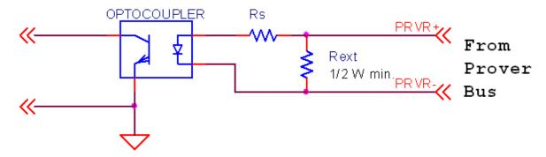
Figure 114: Illustration of using Prover Pulse Bus with Optocoupler
