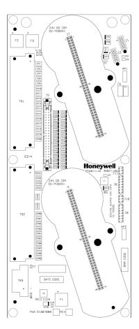
Figure 56: Series C 24V Digital Output 9 inch, redundant IOTA
