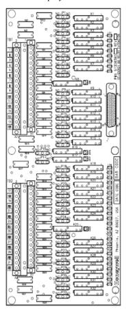
Figure 59: Series C Digital Output Relay Extender board
