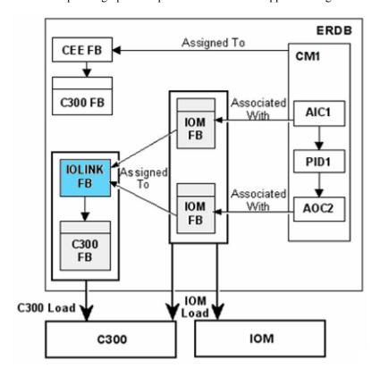
Figure 211: Loading the IOM block the first time
