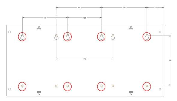
Figure 155: Mounting holes aligned to 13-slot rack
