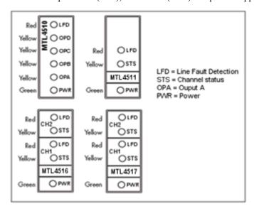
Figure 262: Digital Input - MTL451x isolator LED indicators
