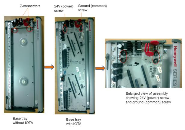
Figure 163: Power connections
