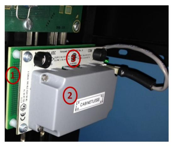
Figure 131: RAM Battery Backup and Battery assembly
