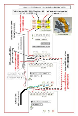
The following figure displays the connection diagram for COTS Power-Meanwell redundant system. The following diagram displays the connection diagram for COTS power-Phoenix redundant system.
