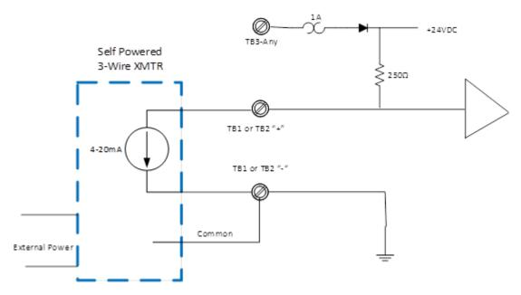
Figure 89: Self-powered 3-wire transmitter with system ground with UIO-2
