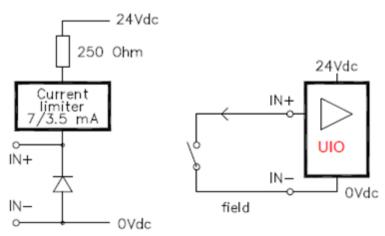
Figure 83: UIO-DI channel configured without open wire detection
