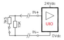
Figure 93: UIO-DI channel configured with open wire detection
