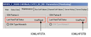
Figure 236: Location of hard failure message
