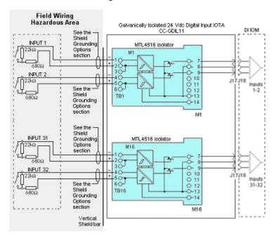
Figure 259: CC-GDIL11 Digital Input IOTA connection diagram
