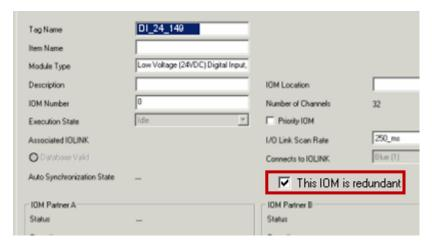
Figure 166: Defining redundancy from the Main tab
