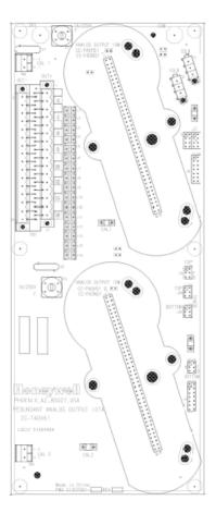
Figure 33: Series C Analog Output 12 inch, redundant IOTA
