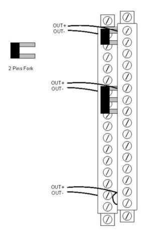
Figure 85: DO channel wiring for ganging
