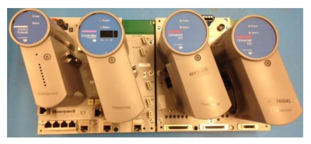
Figure 2: View of Universal Horizontal Input/Output (UHIO)
