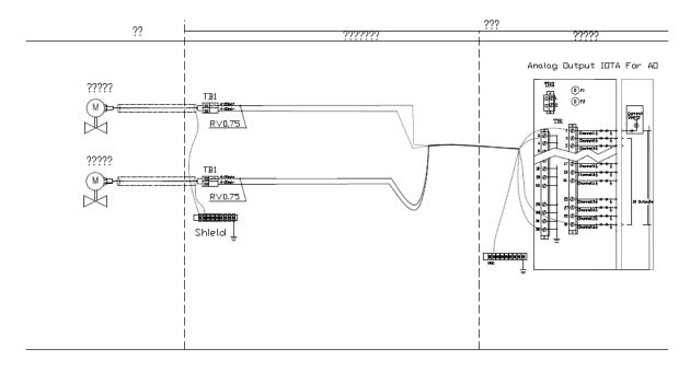
Figure 32: Series C Analog Output 6 inch, non-redundant IOTA and field wiring connection
