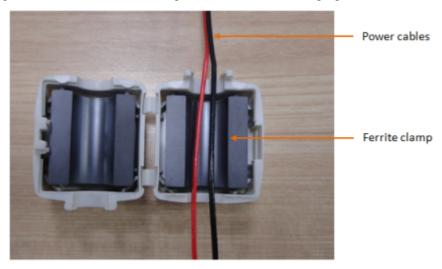
**c** Wind the power cables on the ferrite clamp as shown in the following figure.
