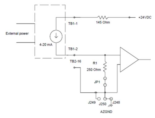
Figure 22: Non-redundant Analog Input 9 inch, self-powered 2-wire transmitter wiring
