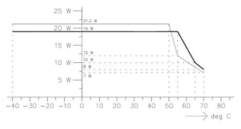
Thick line: applicable for most applications having AO<=20mA and AI<=24mA Thin line: applicable if one or more channels have AO>20mA or AI>24mA
