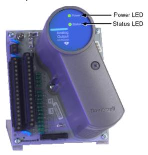
Figure 214: Series C I/O LED indicators
