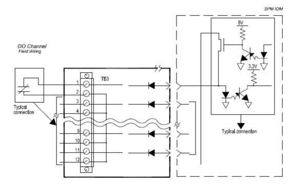
Figure 68: Series C SPM - DO Channel Field Wiring
