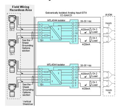
Figure 246: CC-GAIX21 Analog Input IOTA connection diagram
