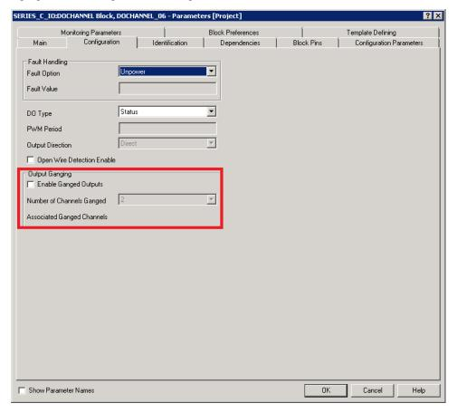
Figure 178: Configuration tab - UIO-DO channel
