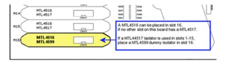
Figure 257: CC-GDIL11 DI and isolator usage
