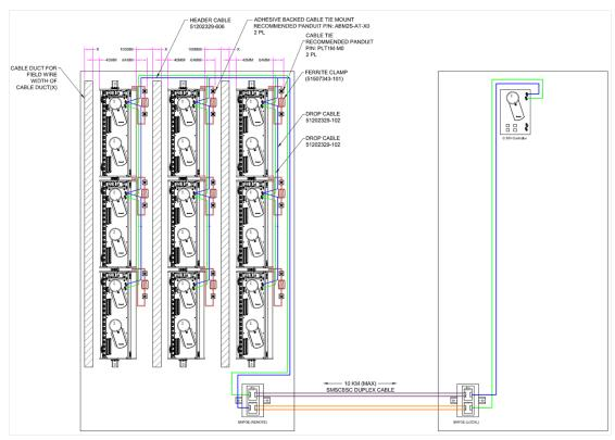
Figure 160: End-to-end system wiring - Rail-UIOs in single cabinet
