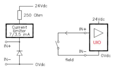
Figure 95: UIO-DI channel configured without open wire detection
