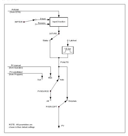
Figure 207: SVP - Digital Input conversion
