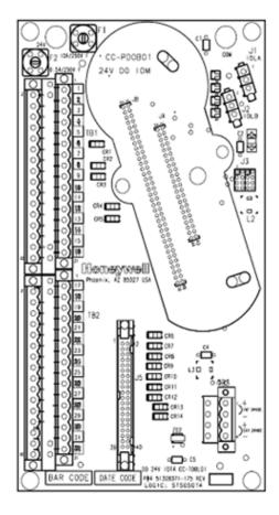
Figure 51: Series C 24V Digital Output 9 inch, non-redundant IOTA
