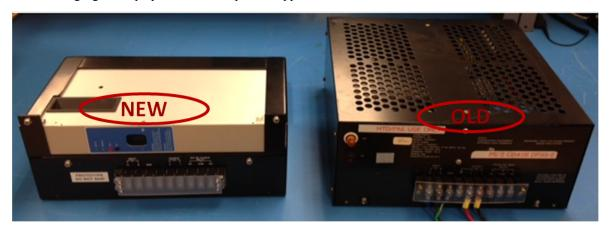
Figure 134: Old and new power supply
