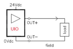
Figure 84: UIO as a Digital Output
