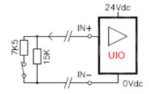
Figure 81: UIO-DI channel configured with open wire detection
