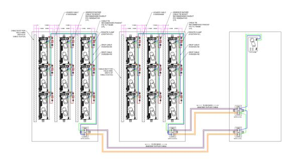
Figure 161: End-to-end system wiring - Rail-UIOs in adjacent cabinet
