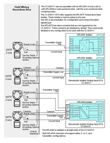
Figure 247: Transmitter Field Wiring to CC-GAIX11/GAIX21 IOTAs
