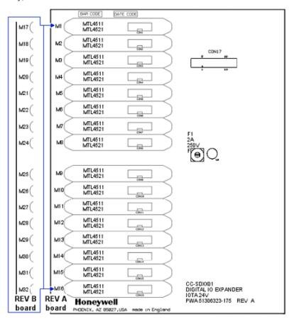
Figure 267: CC-SDXX01 Digital Output IOTA assembly layout
