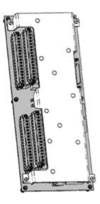
Figure 61: Series C Digital Output Relay Cover
