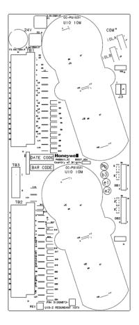
Figure 87: Universal Input/Output Module, 12 inch, redundant IOTA
