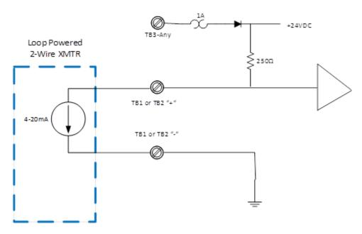
Figure 88: Standard 2-wire transmitter with UIO-2
