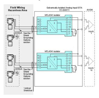
Figure 244: CC-GAIX11 Analog Input IOTA connection diagram
