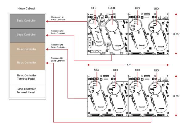
Figure 4: Mapping the CB/EC with the UHIO components
