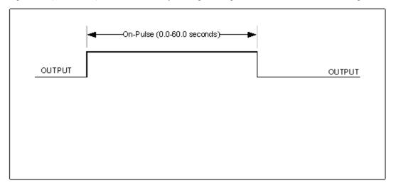
Figure 202: Speed Digital On Pulse Output
