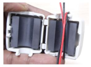
**d** Wind the four turns on the ferrite clamp as shown in the following figure.
