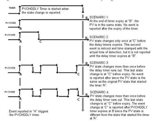
Figure 216: SOE PV Change Delay Scenario
