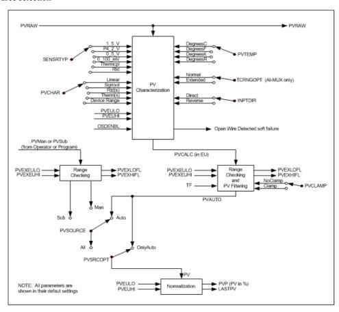
Figure 190: Analog Input conversion
