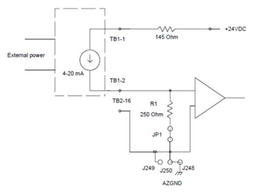
Figure 25: Non-redundant Analog Input 9 inch, self-powered 2-wire transmitter wiring
