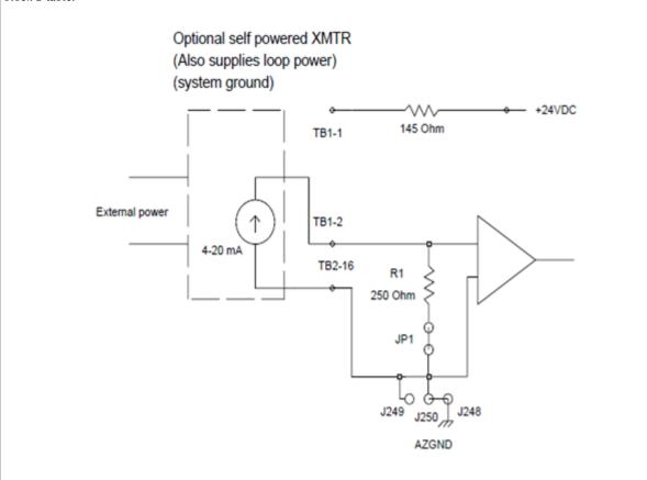
Self-powered transmitter with device grounded
