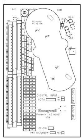
Figure 36: Series C Digital Input High Voltage 9 inch, non-redundant IOTA
