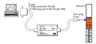
Parameters can be configured, for example sensor type, measuring range and alarm signals. These can then be saved and later used to configure other MTL4575s isolators.
