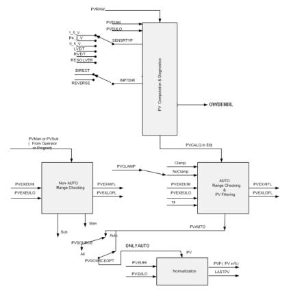
Figure 206: SVP -AI PV processing when it is configured other than LVDT/RVDT or Resolver
