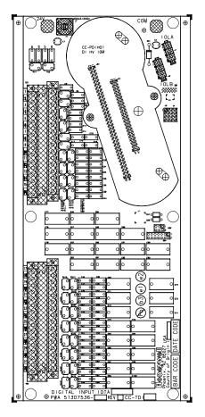
Figure 40: Series C Digital Input High Voltage 12 inch, non-redundant PROX IOTA
