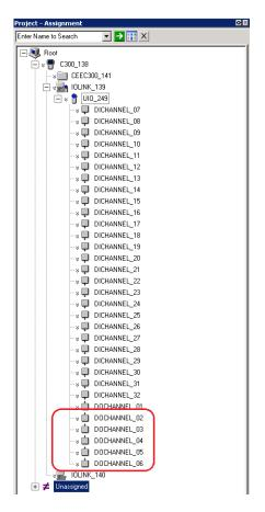
Figure 186: Appearance of DO channels before ganging
