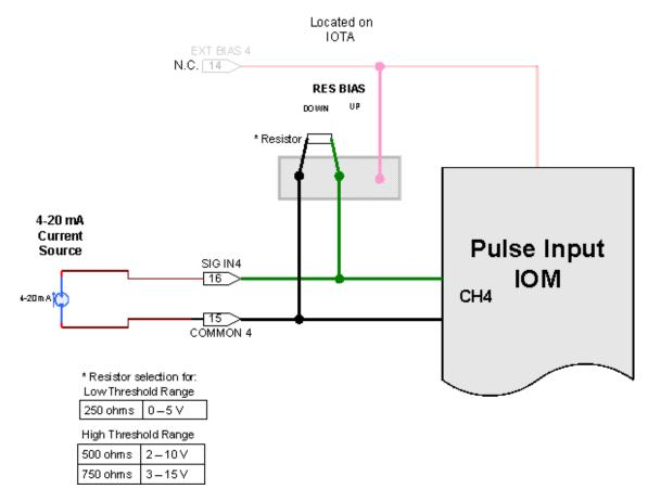
Figure 121: Connecting PIM with a 4-20mA current source
