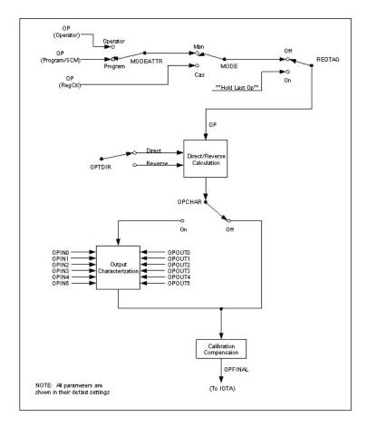
Figure 198: Speed Analog Output conversion
