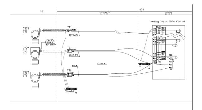
Figure 18: Series C Analog Input 6 inch, non-redundant IOTA and field wiring connection
