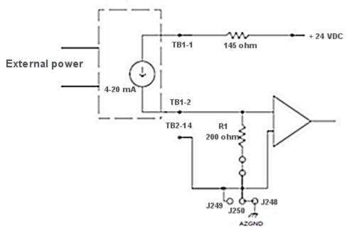
Figure 17: Non-redundant Analog Input 6 inch, self-powered 2-wire transmitter wiring
