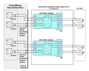
Figure 254: CC-GAOX21 Analog Output IOTA connection diagram
