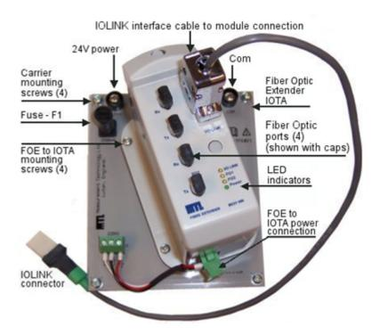
Figure 231: Fiber Optic Extender assembly
