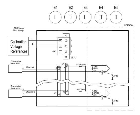
Figure 63: Series C SPM - AI Channel Field Wiring
