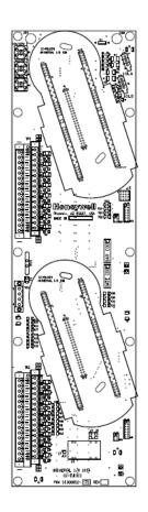
Figure 75: Universal Input/Output Module, 18 inch, redundant IOTA
