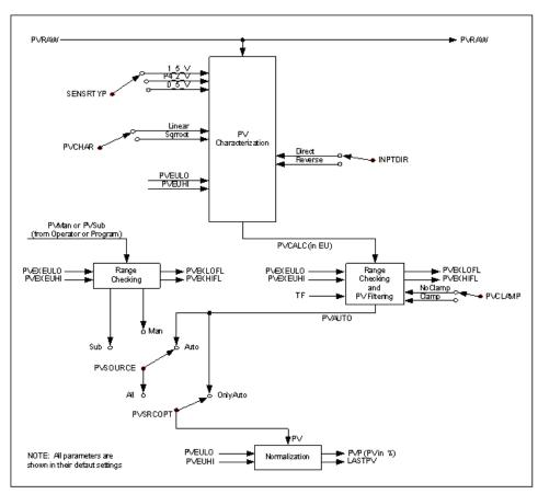
Figure 197: Speed Analog Input conversion
