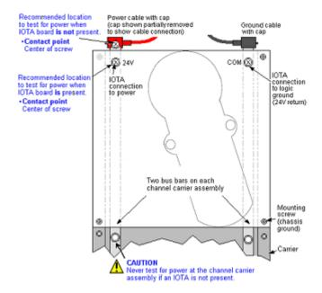
Figure 11: Grounding and power connections
