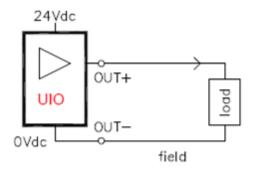
Figure 96: UIO-2 as a Digital Output
