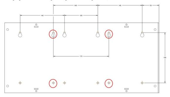
Figure 153: Mounting holes aligned to 7-slot rack
