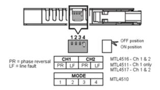
Figure 241: DI module switch setting
