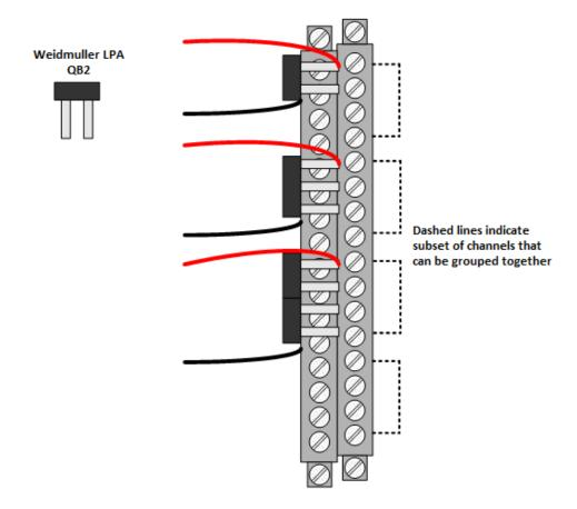
Figure 97: DO channel wiring for ganging
