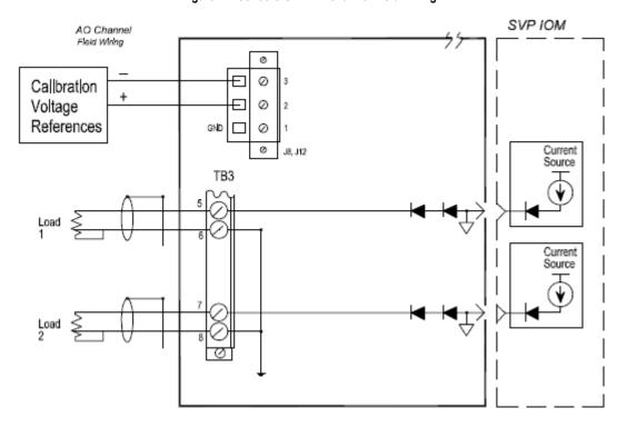
Figure 73: Series C SVP - AO channel Field Wiring
