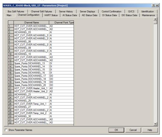
Figure 128: UIO channel configuration in the configuration form
