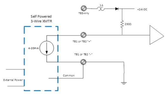
Figure 77: Self-powered 3-wire transmitter with system ground with UIO
