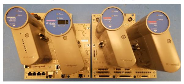
Figure 3: View of Universal Horizontal Input/Output Two (UHIO-2)
