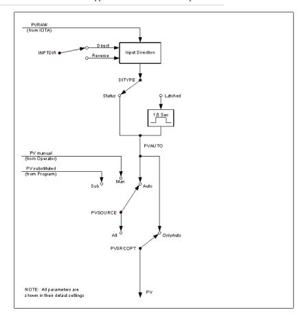
Figure 200: Speed Digital Input conversion
