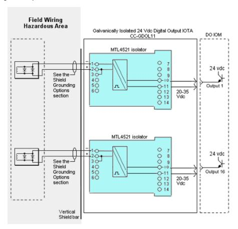
Figure 265: CC-GDOL11 Digital Output IOTA assembly layout
