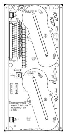
Figure 30: Series C non-HART Analog Input 12 inch, redundant IOTA
