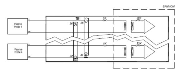
Figure 64: Series C SPM - Passive Probe Field Wiring
