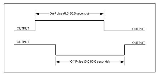
Figure 196: On-Pulse and Off-Pulse Output types
