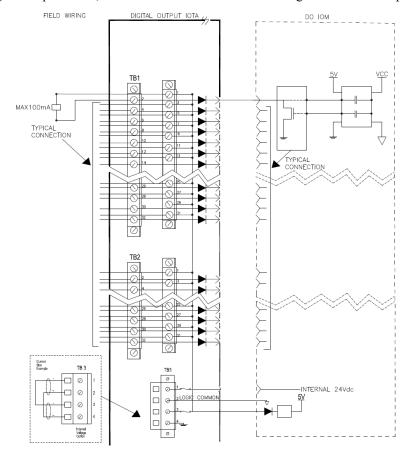
Figure 55: Series C 24V Digital Output 9 inch, non-redundant IOTA and field wiring connections
