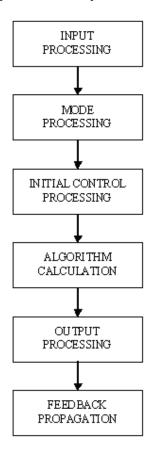
Figure 208: SVP - REGCTL block processing diagram
