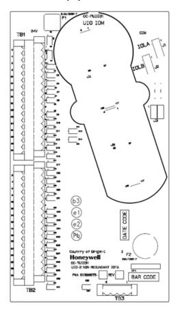
Figure 86: Universal Input/Output Module, 9 inch, non-redundant IOTA
