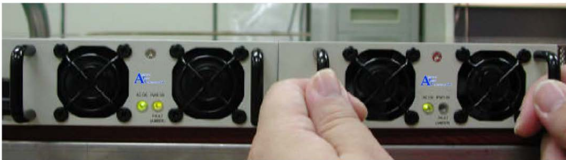
Step 2 : Let the first set of pins contacted and AC OK LED is ON.
