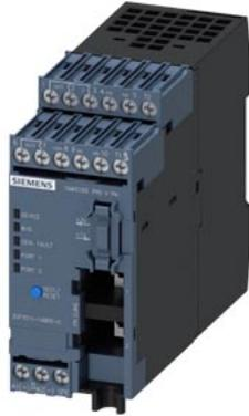
Basic unit SIMOCODE pro V PN, Ethernet/PROFINET IO, PN system redundancy, OPC UA server, Web server, transmission rate 100 Mbps, 2 x bus connection via RJ45, 4I/3O freely parameterizable, Us: 24 V DC, input for thermistor connection
