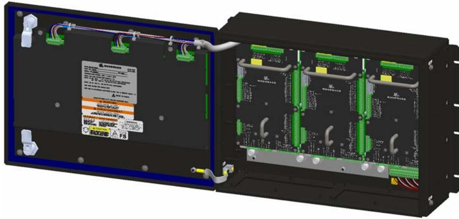
Figure 2-2a. Typical ProTech-GII Bulkhead Package—Front Door Open
